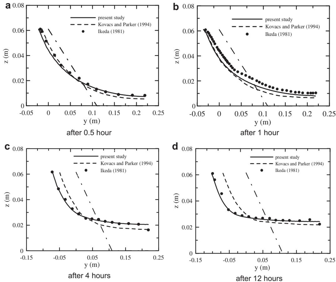
Fig. 5. Change of channel cross section with time.
