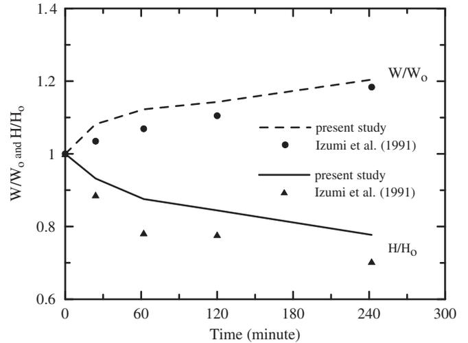
Fig. 9. Change of water surface width and flow depth at the center of the channel (Izumi et al.'s Exp).
