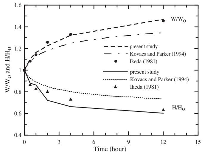
Fig. 6. Change of water surface width and flow depth at the center of the channel (Ikeda's Exp).
