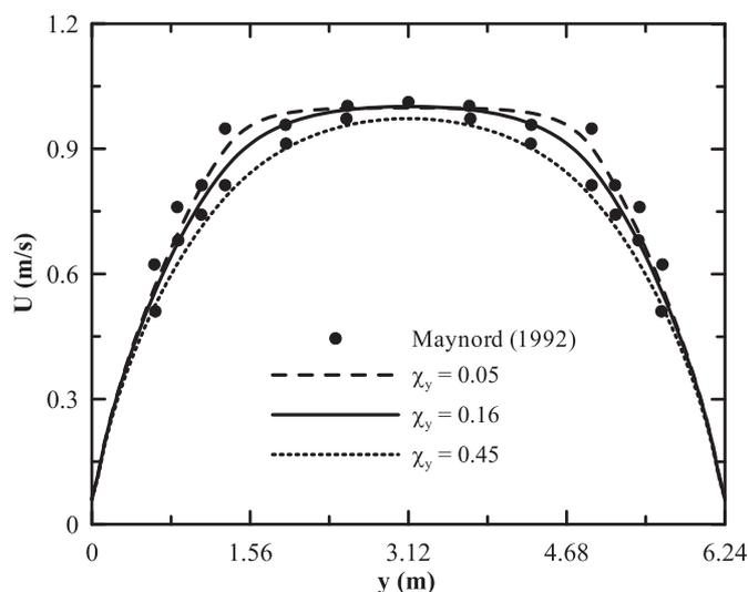
Fig. 4. Impact of non-dimensional eddy viscosity on the depth-averaged velocity.
