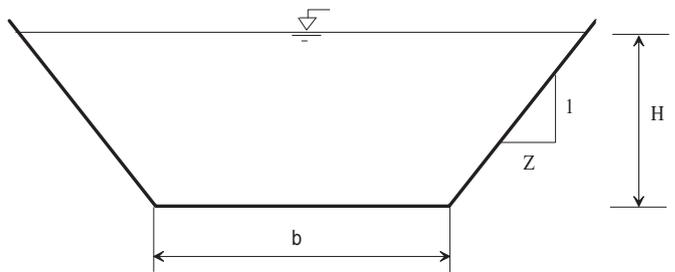
Fig. 2. Schematic sketch of a trapezoidal channel.
