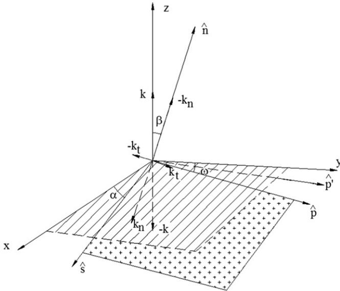
Fig. 1. Coordinate systems used in the sediment transport model in Kovacs and Parker (1994).
