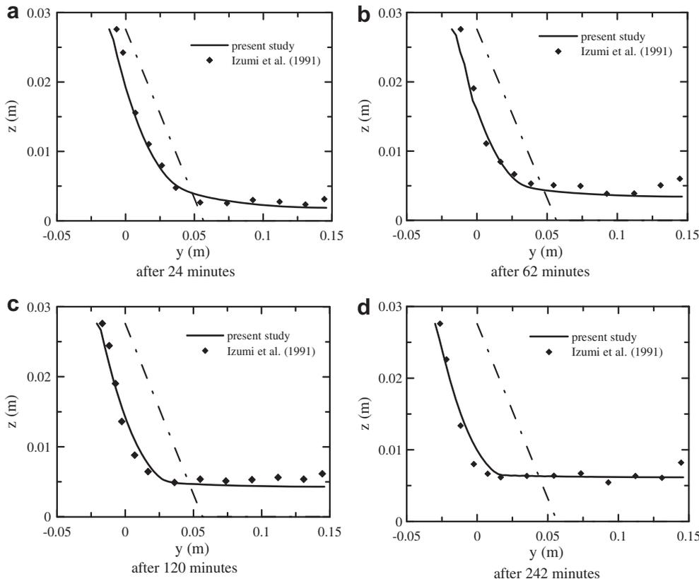
Fig. 8. Change of channel cross section with time.
