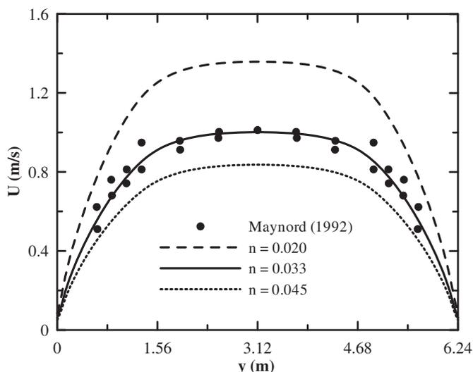
Fig. 3. Impact of roughness coefficient on the depth-averaged velocity.
