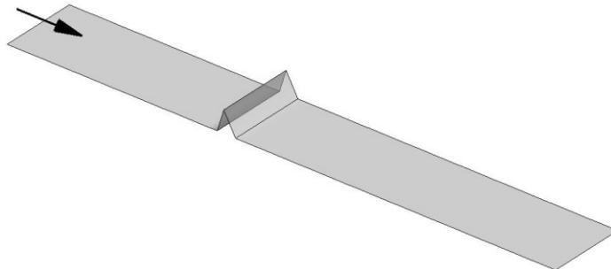
Figure 2 Initial bed profile with a triangular hump
