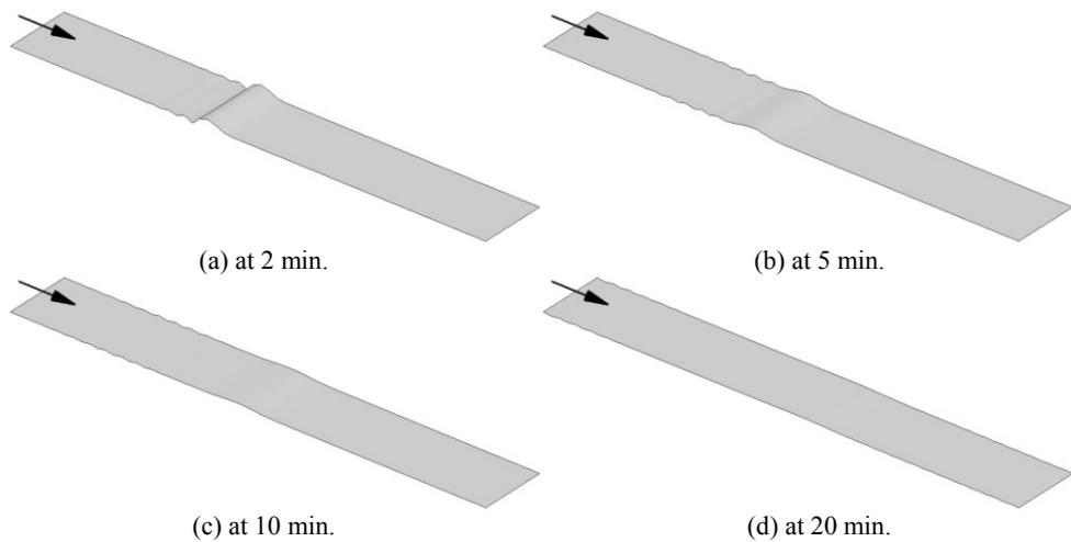
Figure 4 Bed elevation change simulated by downwind weighting scheme
