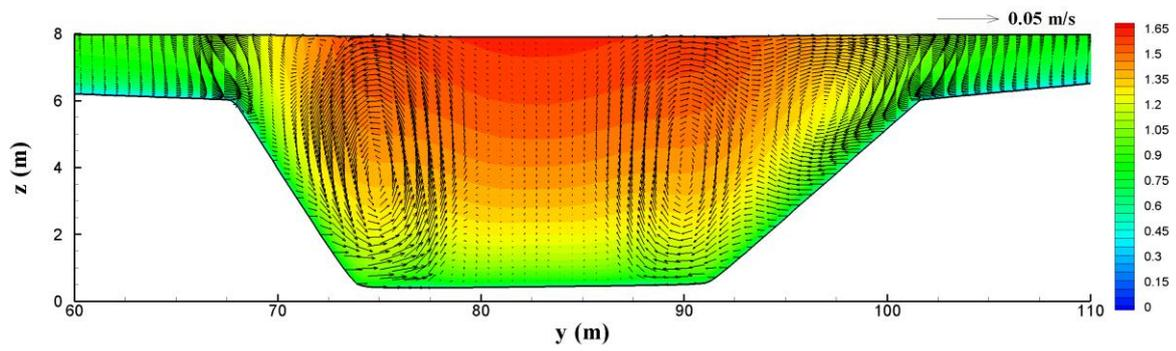
**Figure 3. Streamwise mean velocity with secondary current vectors (unit, m/s)**
