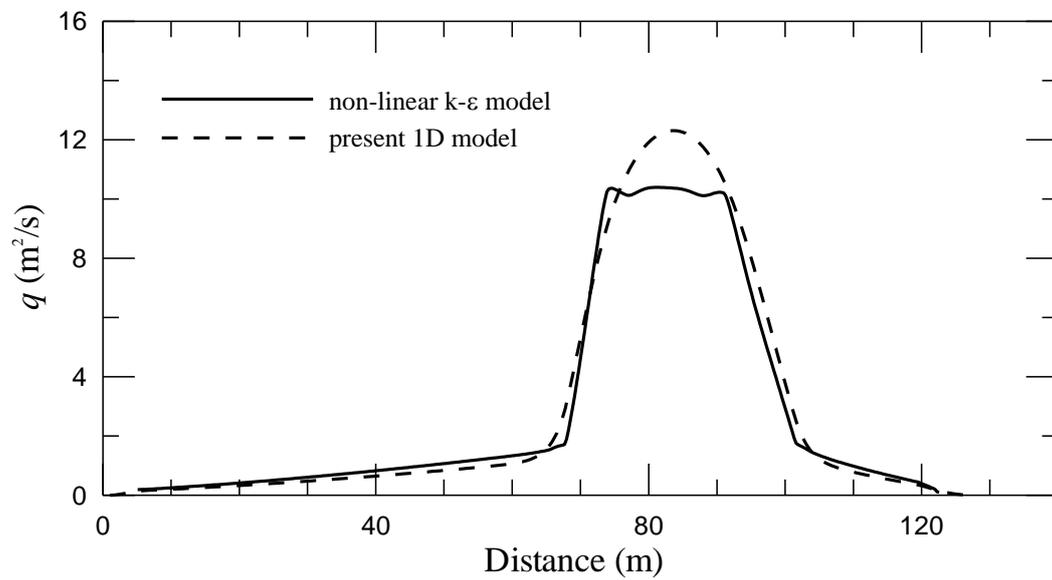
**Figure 4. Lateral distribution of the unit discharge in the Severn River in UK**
