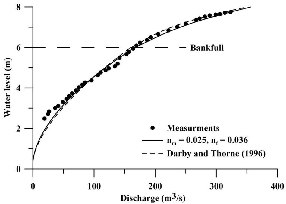
Figure 2. Stage-discharge curve in the Severn River, UK (Choi and Shin, 2009)
