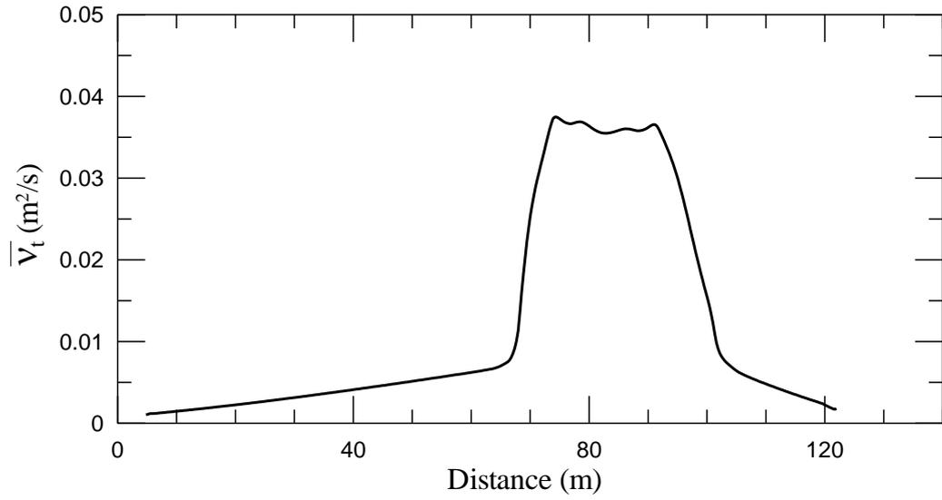
**Figure 5. Lateral distribution of depth-averaged eddy viscosity ( $\bar{v}_t$ )**
