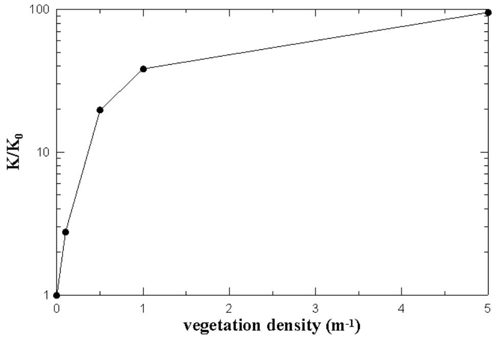
Figure 4. Change of longitudinal dispersion coefficient with vegetation density ( $b_v/b = 0.3$ )
