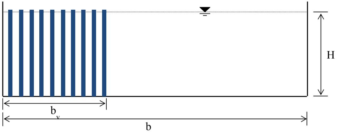
Figure 2. Schematic sketch of partly-vegetated open-channel flows
