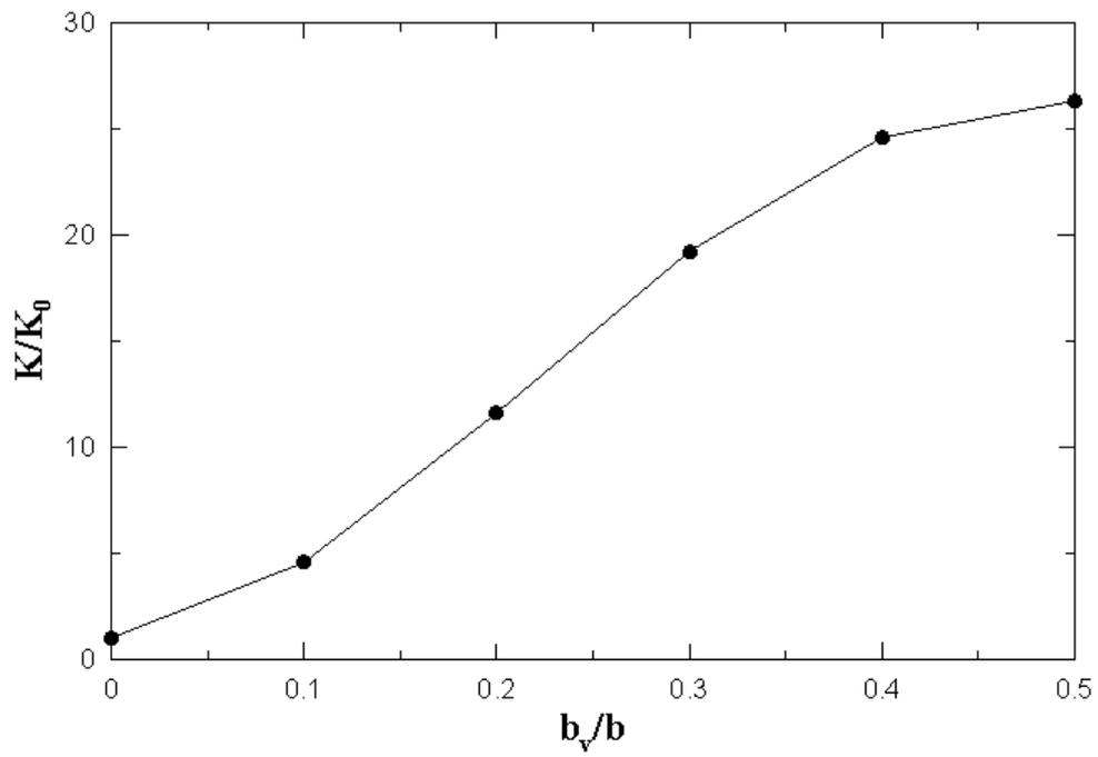
Figure 5. Change of longitudinal dispersion coefficient with width ratio ( $a = 0.5 m^{-1}$ )
