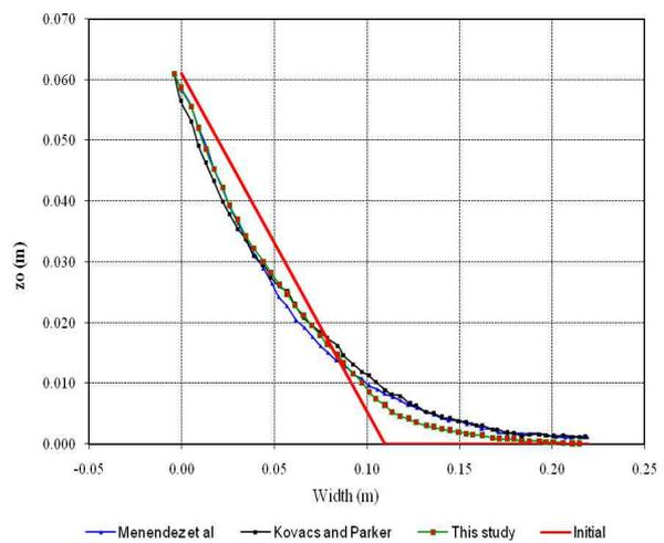
Figure 3. Change of cross section at 404 seconds.
